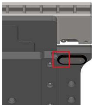
This bump stop has the long end pointing inwards. Flipping it will increase the travel limit by 5 mm.
